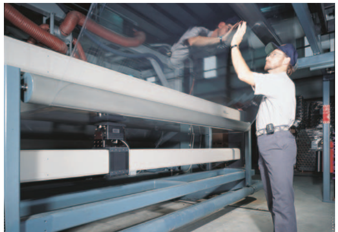
Sensor and scanner assembly for measurement of film
