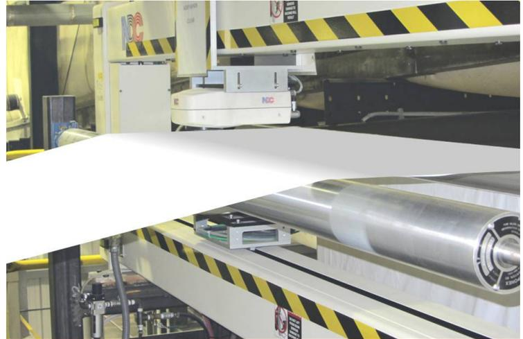
FG710S Infrared Transmission Sensor
